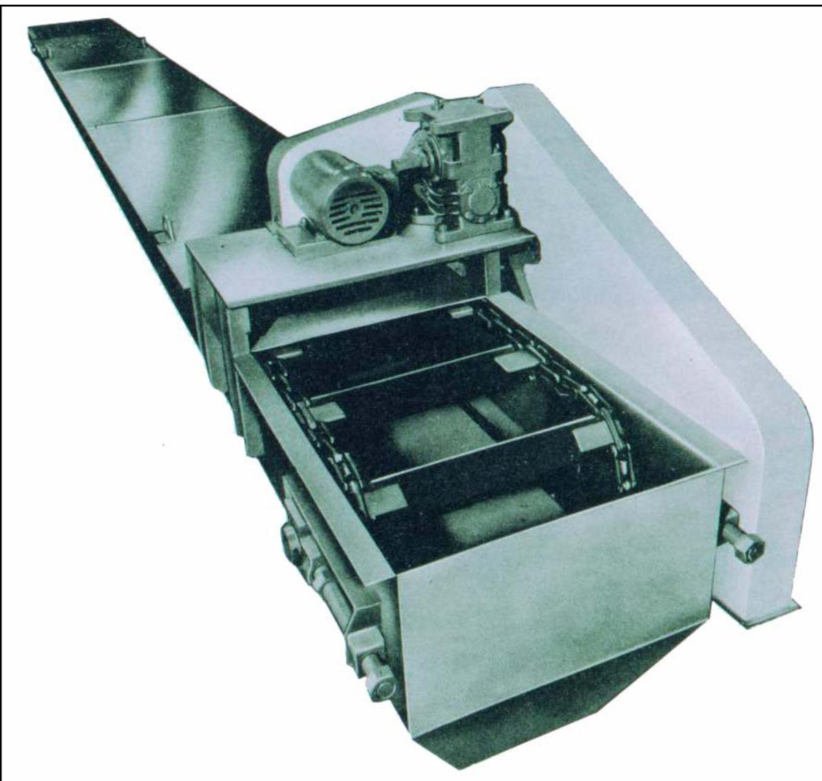
**The chain manufactured with forged links
